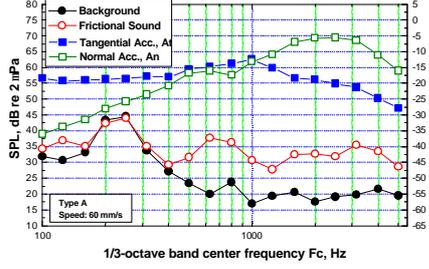
Fig. 8 1/3-octave spectrum of sound and acceleration. Type A fixing
