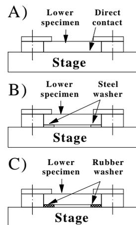
Fig. 3 Types of lower specimen fixation
