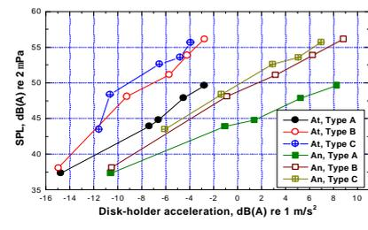
Fig. 6 Relation between tangential and normal acceleration levels and sound pressure level (SPL)
