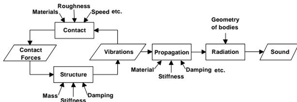
Fig. 1 Concept of frictional sound generation
