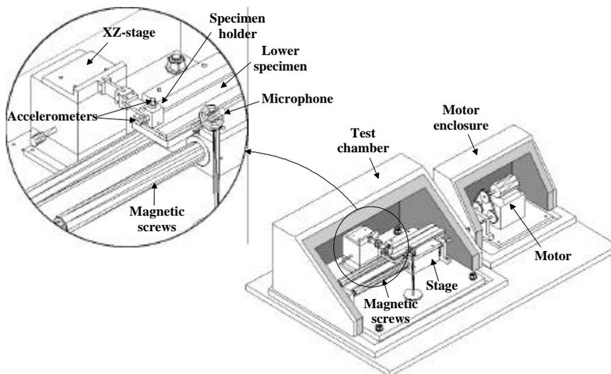
Fig. 2 Experimental Apparatus
