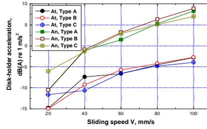
Fig. 5 Effect of sliding speed on tangential and normal acceleration levels of disk-holder.
