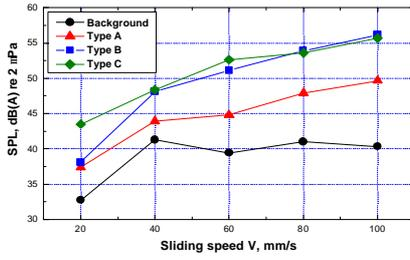
Fig. 4 Effect of sliding speed on sound pressure level (SPL)
