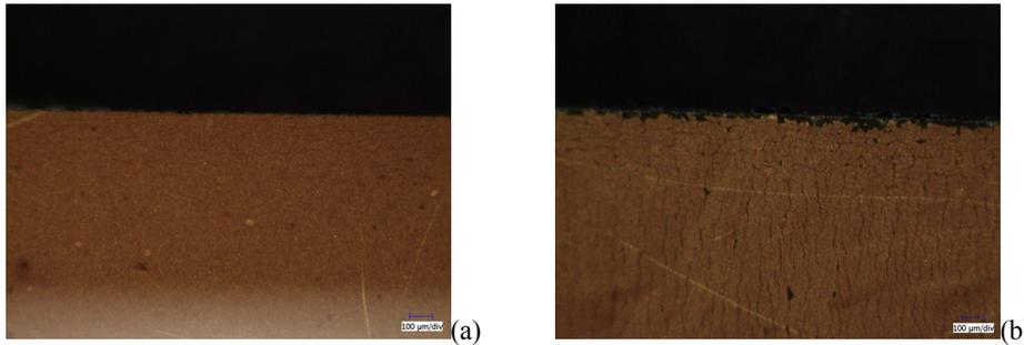
Fig.3. Optical microscope images of the electrode surface of a “just made” (a) and “well worked” (b) IPMC.
