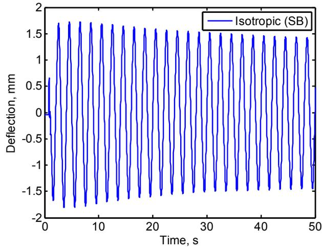
Fig.10. Deflection of IPMC (gold plated Nafion 1110, 40 x 4 mm, 285  $\mu\text{m}$  thickness) with isotropic surface under excitation by 1 V 0.5 Hz sine voltage.
