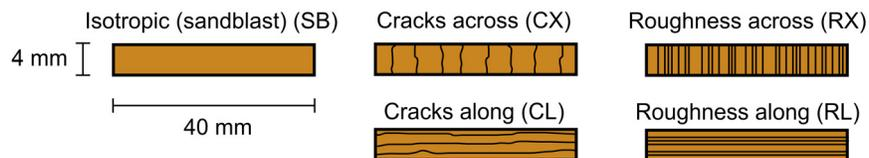
Fig. 7. Schematic drawing of the 5 IPMC specimens used in the tests.
