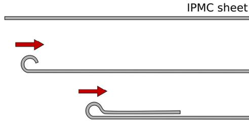
Fig. 4. Forming cracks on the electrode surface by tightly bending and rolling the IPMC.
