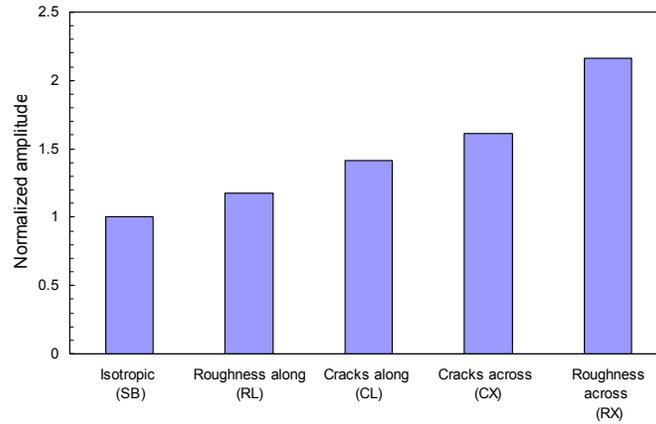
Fig.12. Normalized amplitude comparison for IPMC (gold plated Nafion 1110, 40 x 4 mm, 285  $\mu\text{m}$  thickness) with different surface modifications.
