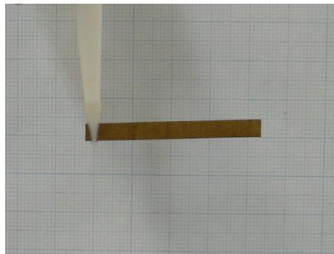
Fig.13. Thick (285  $\mu\text{m}$ ) IPMC with roughened surface is sufficiently rigid in the plane of loading and can easily sustain its own weight.
