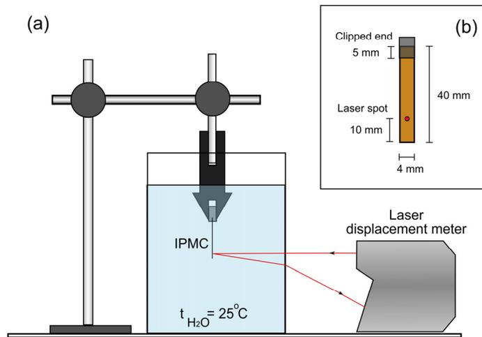
Fig.8. Experimental setup - (a) general view; (b) details of IPMC specimen fixing and measurement spot location.
