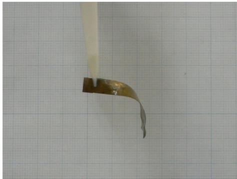
Fig. 1. Thin (60  $\mu\text{m}$ ) IPMC film buckles and twists under it own weight.
