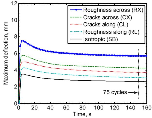
Fig.11. Maximum deflection of IPMC (gold plated Nafion 1110, 40 x 4 mm, 285  $\mu\text{m}$  thickness) with different surface modifications under excitation by 1 V 0.5 Hz sine voltage.
