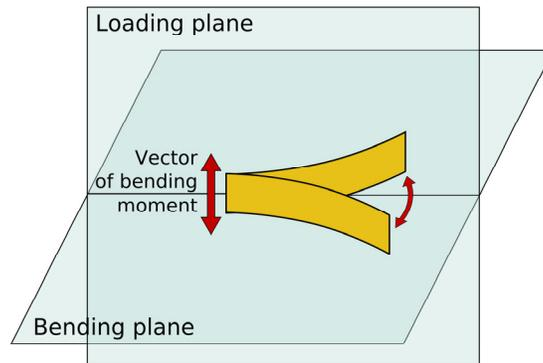
Fig.2. The planes of bending and loading when IPMC is used to propel a swimming robot.
