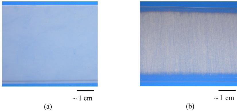
Fig. 5. Nafion 1110 (250  $\mu\text{m}$  thickness) surface after (a) sandblasting, and (b) directional roughening by sandpaper with grain size 240.
