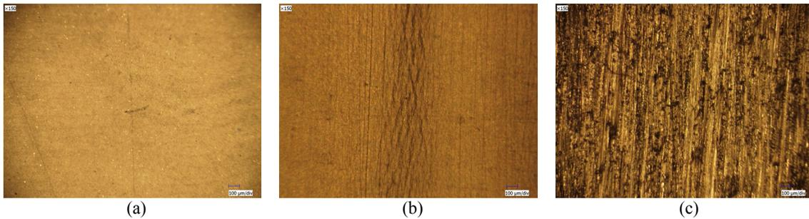
Fig. 6. Optical micrographs of different electrode surfaces of IPMCs. (a) gold plating over sandblasted Nafion surface; (b) artificially introduced mechanical cracks after each plating cycle on sandblasted Nafion surface; (c) gold plating over directionally roughened Nafion surface.
