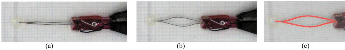
Fig. 16 Activating a pair of linear actuator strips
