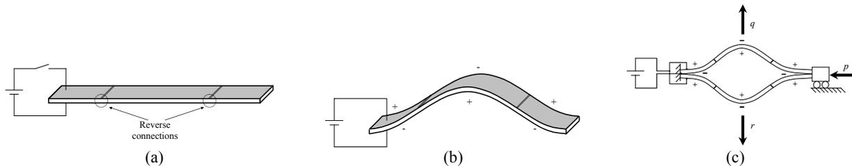
Fig. 11 Three segment linear actuator element
