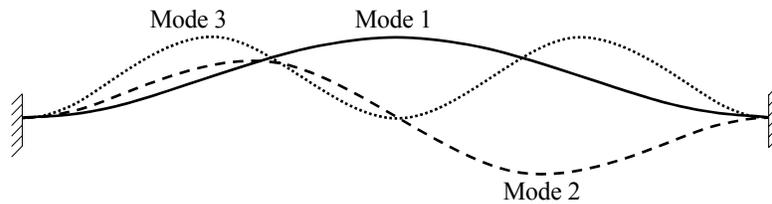
Fig. 6 The first three buckling modes
