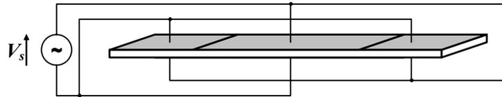
Fig. 9 Electrical connections to a three segment bending actuator
