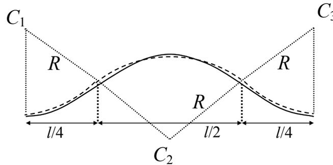
Fig. 7 Three distinct sections in a buckled beam
