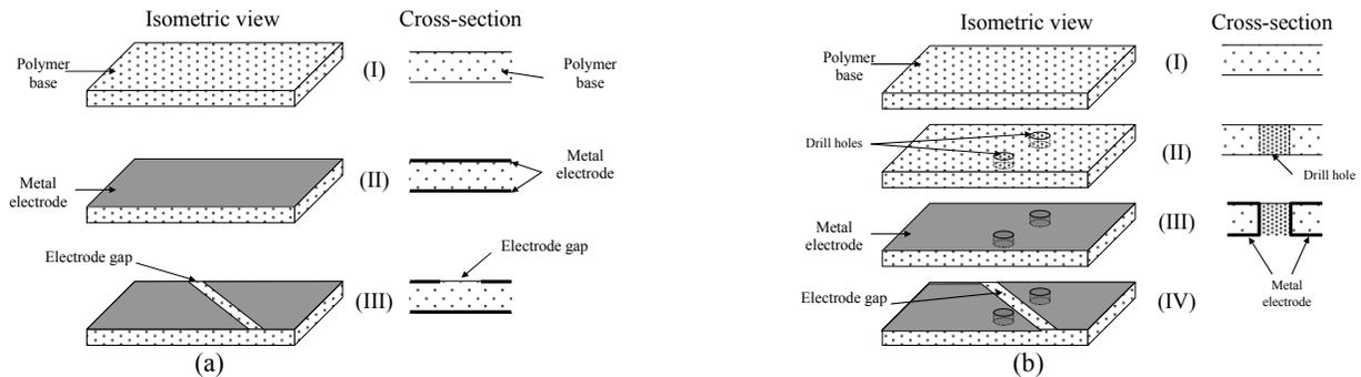
Fig. 12 Manufacturing a polymer-metal composite actuator
