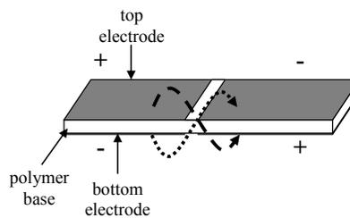
Fig. 10 Reverse connections schema for adjacent segments
