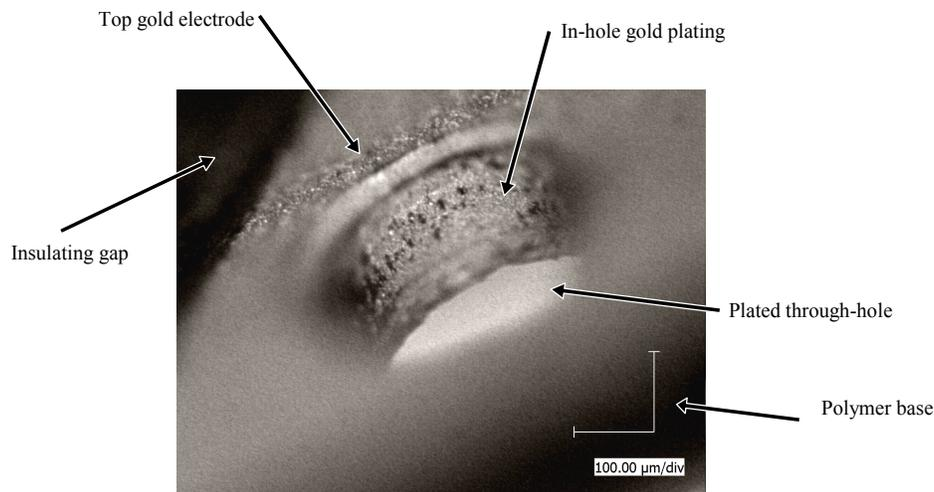
Fig. 13 Microscope picture of plated through-hole
