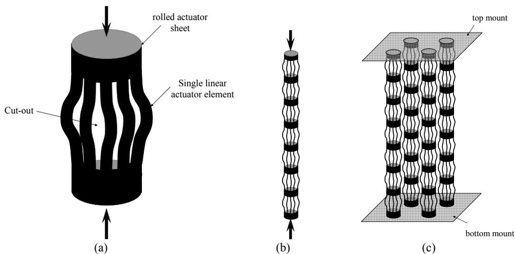
Fig. 19 A cylindrical linear actuator
